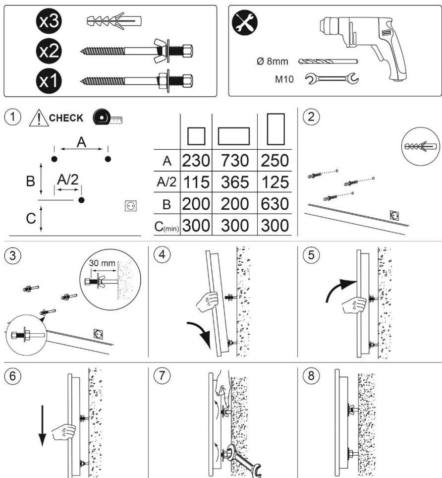
**⚠** Check measures and levelling before drilling. Measurements in mm
