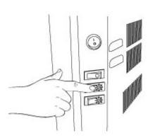
• If you select after this, the first switch below the round shape one, we will have all the switchers connected, this will provide 2000 W.
