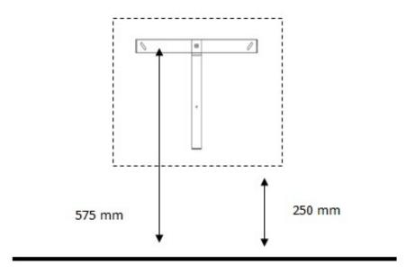
⚠ Check dimensions and level before drilling. ⚠ Dimensions in mm.
