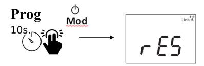
Do not forget to press "MOD" to confirm the reset
